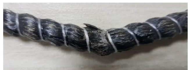
Figure 5: Typical Failure Mode of BFRP Bars in Flexure
