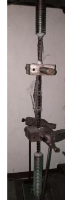
Figure 3: Typical Failure Mode of BFRP Bars in Tension
