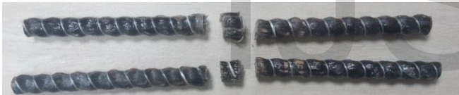
Figure 7: Typical Failure Mode of BFRP Bars in Transverse Shear
