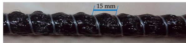
Figure 1: Surface Configuration of the BFRP Bars
