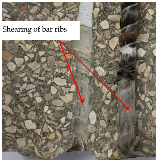
Figure 11: Typical Failure Mode of BFRP Bars in Pull-out
