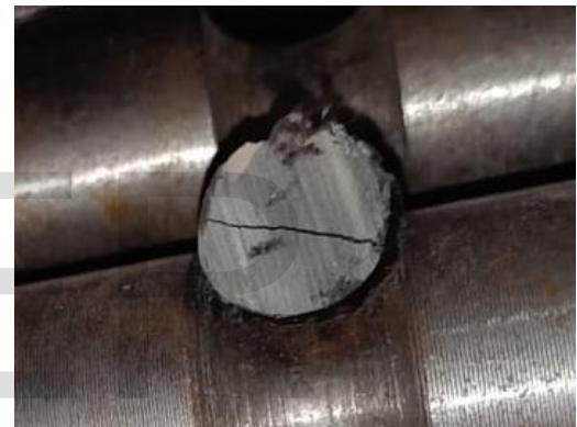
Figure 9: Typical Failure Mode of BFRP Bars in Interlaminar Shear
